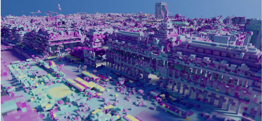
Figure 2.5.: Visualization of a voxelized LiDAR point cloud of the city of Rennes. Points are rearranged in a regular 3D grid, the intensities are averaged in each cell.
